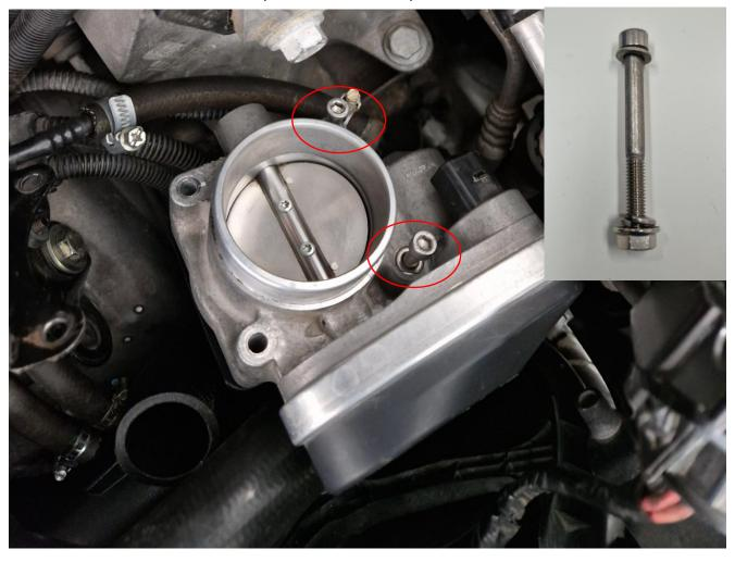
7. Let a bit lose the throttle body bracket. Like the photo above, install two bolts to secure the throttle body to the charge pipe. At this stage do not torque the bolts. The assembly should be loose.
