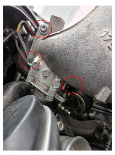
4. Remove the intercooler horn. The horn is secured by three nuts. \*Photo for reference.
