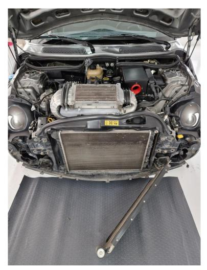
2. Remove the bolts that secure the AC radiator. Carefully put AC radiator aside and pull the plastic shroud that supports the water radiator.
