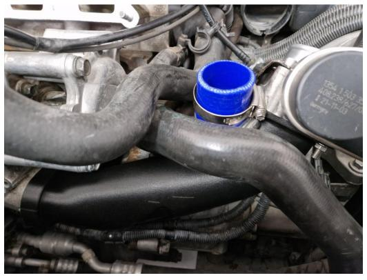
10. Install the bypass hose. Let the hose clamp loose until you secure the intercooler horn.
